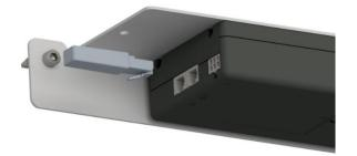
After the Bluetooth adapter has been inserted, it will blink blue and is ready for pairing
