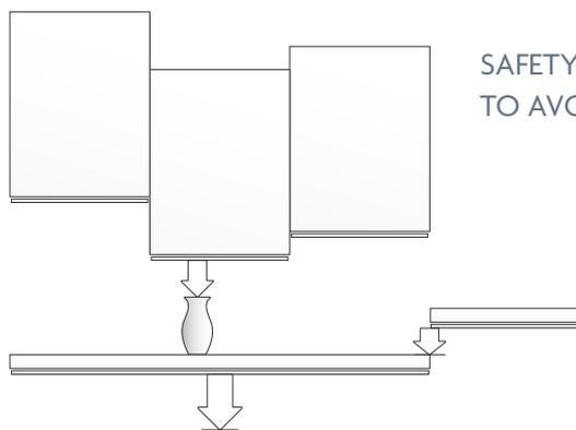
SAFETY STOP INSTALLED TO AVOID TRAPPING
