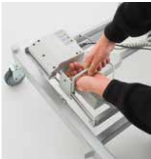
The scissor is released from the base with the quick release handle.
