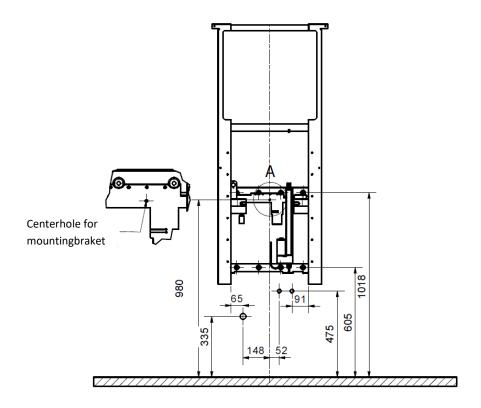
Place the unit in accordance with the water connection and drain as shown on the drawing.
