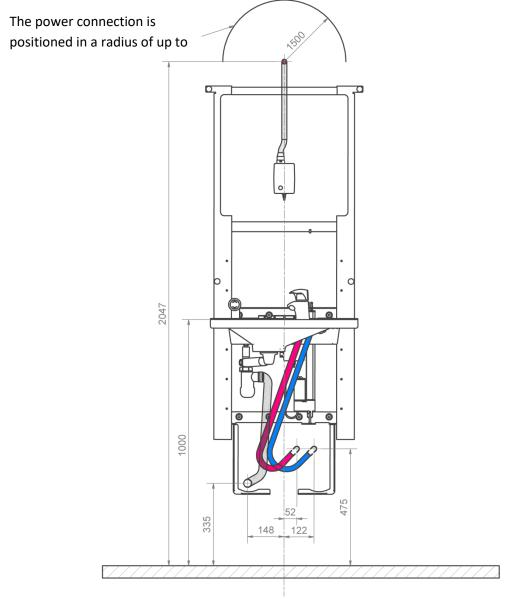
Install water connection and drain hoses as illustrated. Put the installation cover back on. Make sure that all hoses move freely and unhindered.
