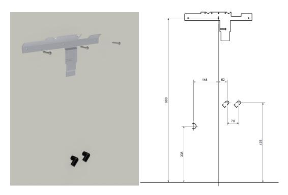
Fix the mounting bracket as illustrated on the drawing with the right distance to water and drain. Make sure that the mounting bracket is level.
