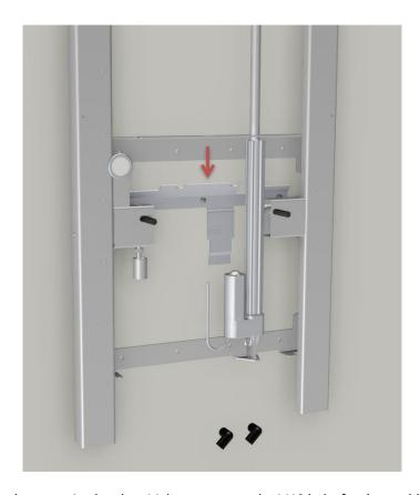
Hang the lifting unit on the mounting bracket. Make sure to put the M12 bolts for the washbasin in the frame prior to mounting.
