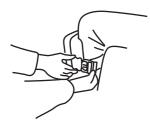
Raise the lifting boom to gain tension on the sling – *Ensure that the sling is still* secure and attached before continuing with the lift.
