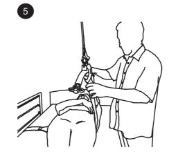
Mount the lifting straps on the lifting hanger of a ceiling hoist or a mobile hoist.
