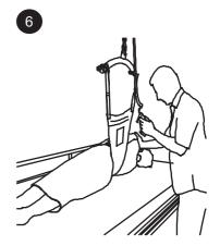
Activate the hoist and support the patient's shoulder at the same time. Never raise the lifting hanger higher than necessary.
